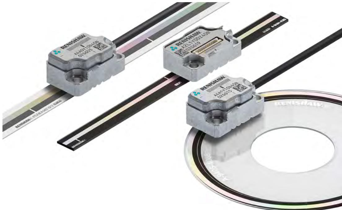
**The ATOM DX™ encoder series is Renishaw's smallest incremental optical encoder with digital output direct from the readhead, providing positional feedback, onboard interpolation, and filtering optics all in a miniature package.**
